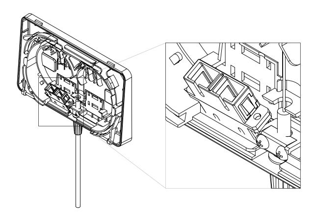
29. INSERT THE SC DUPLEX ADAPTER FROM THE INSIDE OF THE MODULE. ANGLE THE ADAPTER AN INSERT THE END WITHOUT THE METAL CLIP INTO THE SC ADAPTER PORT SO THAT IT PROTRUDES THROUGH THE PORT. THEN LAY THE ADAPTER FLAT AND PUSH IT INDISDE THE MODULE UNTIL THE METAL CLIPS SNAP ONTO THE PLASTIC WALL OF THE MODULE.
