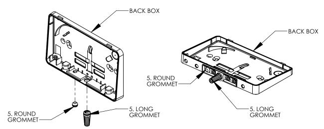
5. IF BOTH CABLES ENTER THROUGH THE BOTTOM SURFACE OF THE BACK BOX, THEN INSERT THE ROUND GROMMET INTO THE CABLE PORT, WHICH WAS KNOCKED OUT. INSERT THE LONG GROMMET INTO THE CENTER CABLE PORT, WHICH IS PROVIDED OPEN.
