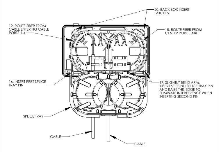
16 INSERT ONE OF THE TWO SPLICE TRAY PINS INTO ONE OF THE TWO HOLES LOCATED IN THE BACK BOX INSERT.
