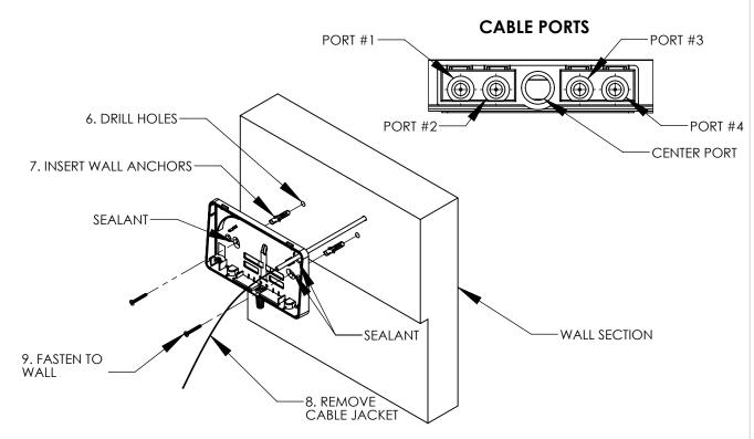
6. FOLLOW SAFETY GUIDLINES AND LOCAL PRACTICES WHEN DRILLING HOLES INTO AN UNFAMILIAR WALL. DRILL TWO .295" (7.5MM) OD X 1 1/4" (31.75MM) DEEP HOLES FOR THE WALL ANCHORS. IF REQUIRED, THE THIRD HOLE IS FOR THE CABLE. SIZE THE CABLE HOLE SO THAT IT EASILY PASSES THROUGH THE WALL.
